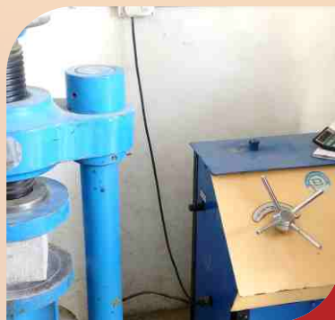
Testing compressive strength of every batch lot before providing to site
